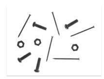
2 The image is thresholded into a region (a run-length encoded binary image) and then split into connected components:
